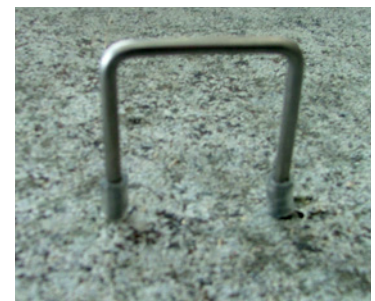
Omega clip in granite. Source: M. E. Hachborn Engineering
