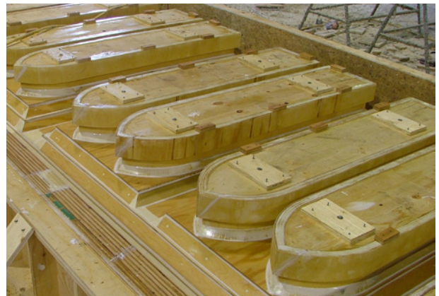
Manufacture of custom wood form used to make precast panels.
