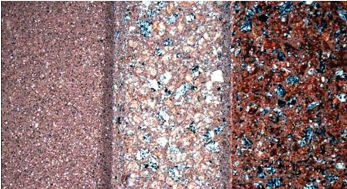
Depth of sandblast or acid etching can produce distinct colours. Source: CPCI
