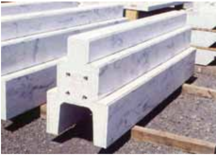
Marble faced precast concrete fins are 3 x 6 feet x variable length.
