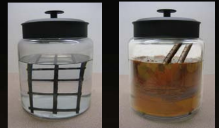
C-GRID reinforcement in CarbonCast products is not susceptible to corrosion like conventional steel mesh reinforcement.
